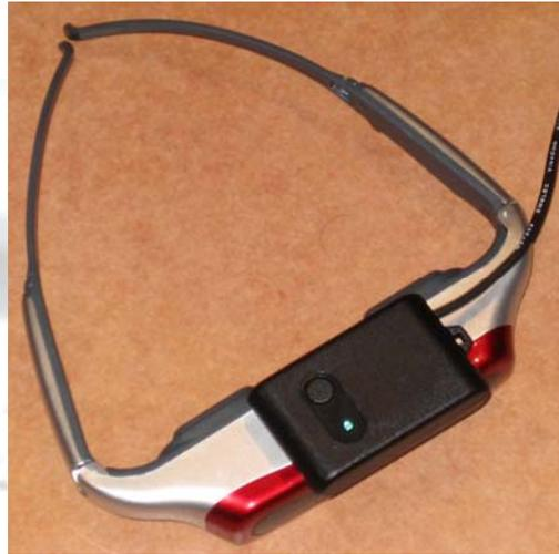
Place the Head Tracker completely horizontal on your cap/glasses and be sure it will not be moved by the cables action.
