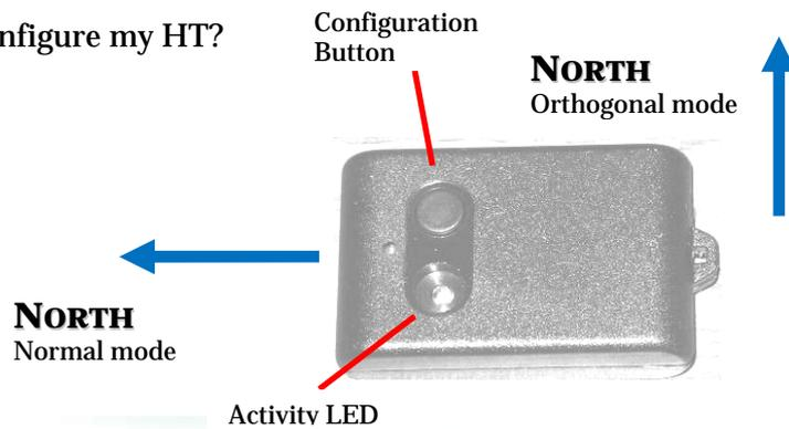
To enter to the configuration mode you have to press the config button during at least ½ second and no more than 2 seconds.
